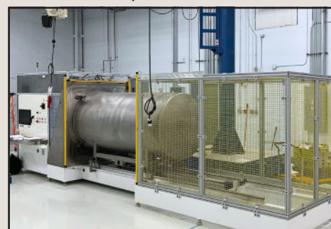
787 SCU/CRU Helium Leak Station
